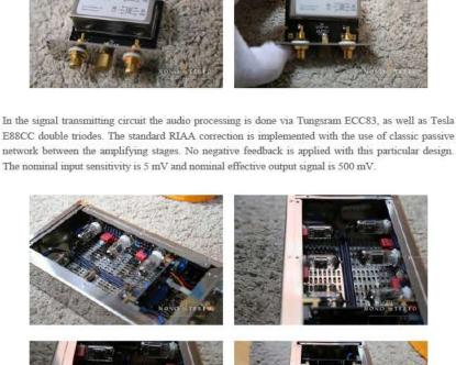
The interior of the device has a unique thermal design for optimal cooling and shortest signal path. In order to achieve the lowest possible noise level Audio Hungary team have separated the power supply from the main phono chassis.
